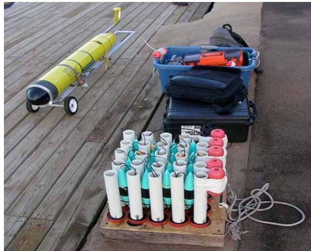
Figure 4 (U) Slocum AUV with multi-element towed array in storage (from SSC)
