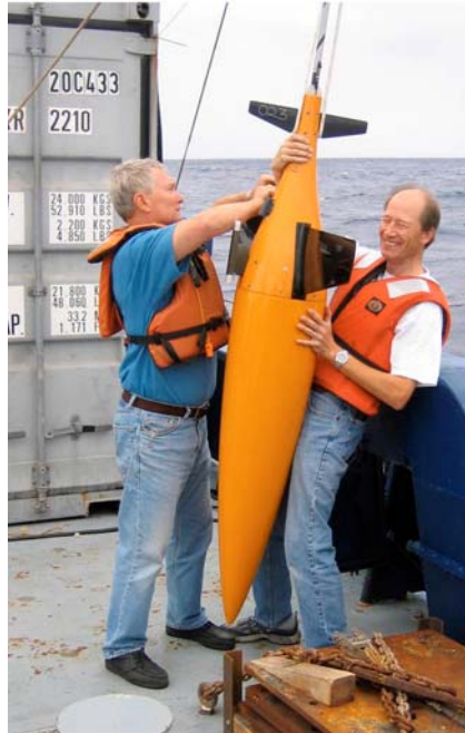
Figure 3 (U) Seaglider AUV during shipboard recovery (from APL-UW)
