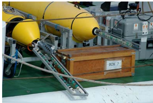
Figure 2 (U) Bluefin-21 AUVs showing single and dual linear nose arrays (above) and array towing assembly model (from Bluefin Robotics, Inc.) (below)
