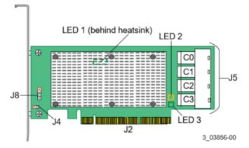
The following table describes the connectors on the HBA 9405W-16i Tri-Mode storage adapter.
