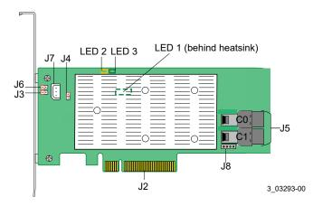
The following table describes the headers and connectors on the MegaRAID 9440-8i Tri-Mode storage adapter.
