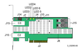
The following table describes the headers and connectors on the MegaRAID 9480-8i8e Tri-Mode storage adapter.
