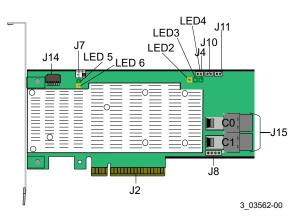
The following table describes the headers and connectors on the MegaRAID 9460-8i Tri-Mode storage adapter.
