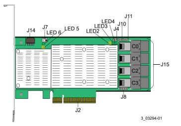
The following table describes the headers and connectors on the MegaRAID 9460-16i Tri-Mode storage adapter.
