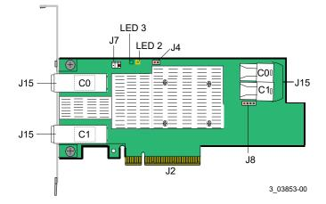
The following table describes the headers and connectors on the HBA 9400-8i8e Tri-Mode storage adapter.
