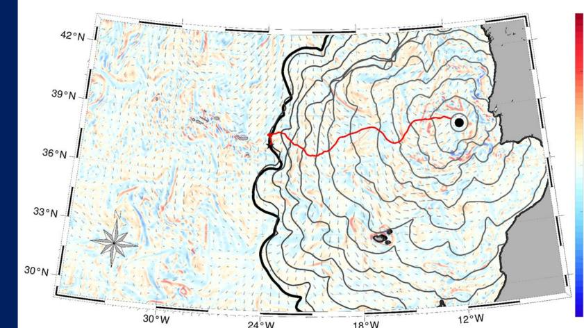
Surface Craft Lisbon to Azores: Time-Optimal path for a surface craft travelling from offshore Lisbon to offshore Azores with a vehicle speed of 0.5 m/s (~1 knot). For this period, our datadriven ocean modeling and optimal path planning predict that the journey will take 23.4 days.
