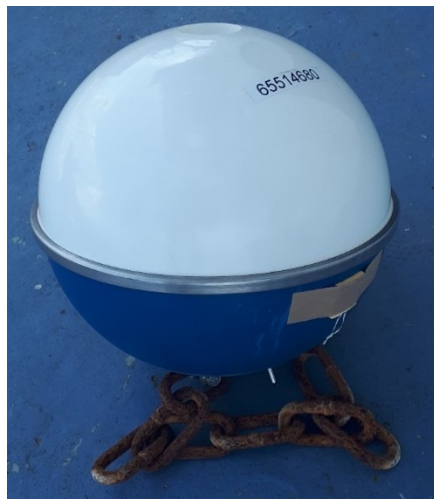
Figure 8: DWS drifter (surface buoy with ballasting chain)
