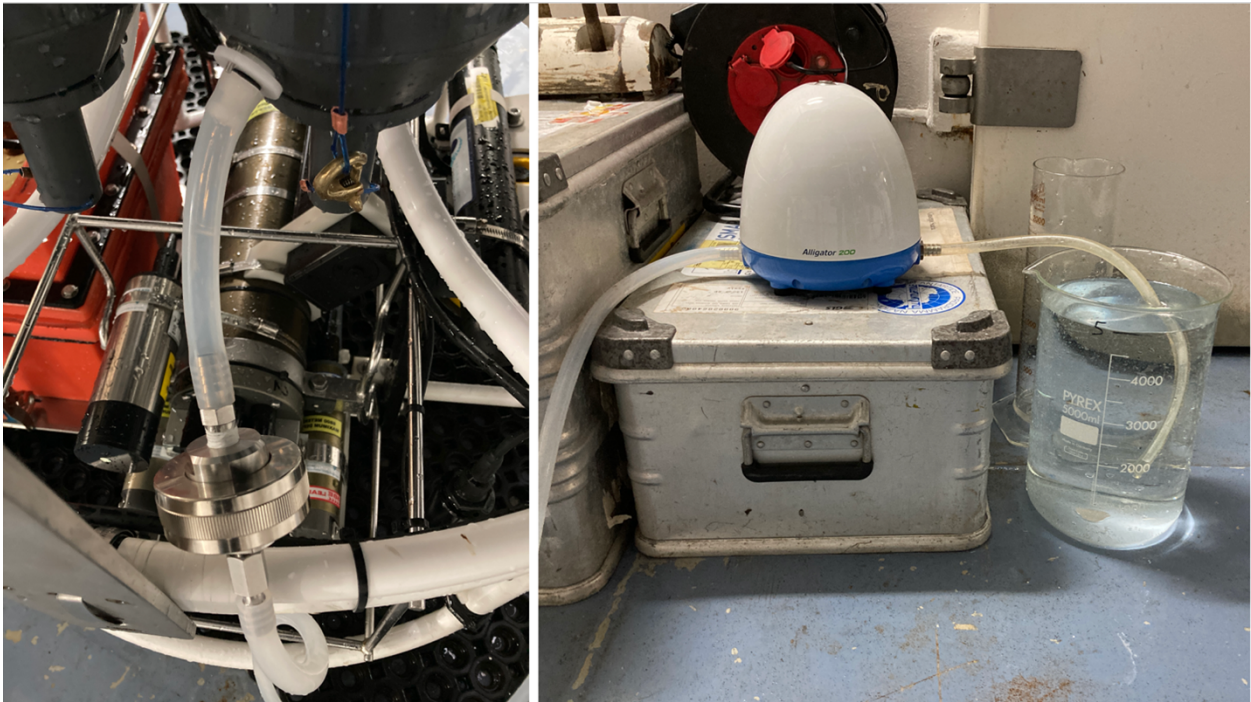
Figure 55: Microplastic sampling set-up at CTD stations. Once on-board the Niskin's bottle faucet is directly connected to a 47mm stainless-steel filter-holder. Seawater is filtered using a diaphragm liquid vacuum pump and the filtered volume is measured using graduated glass cylinders collecting seawater outflow from the pump.
