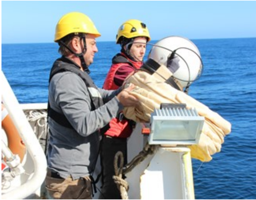
Figure 16: Deployment of a SVP drifter from the stern of the ship.
