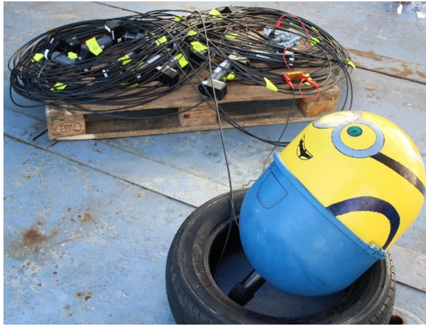
Figure 9: ADOS drifter (surface buoy with thermistor chain)
