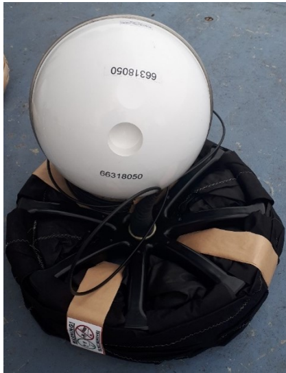
Figure 7: SVP drifter (surface buoy and folded holey sock drogue)
