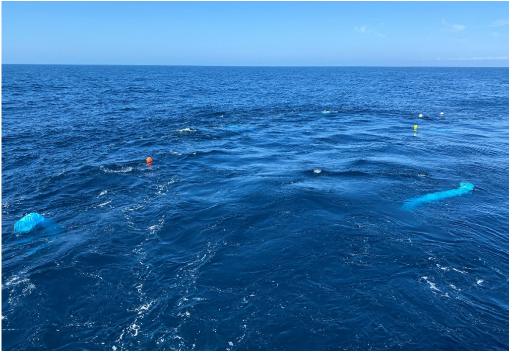
Figure 38: Drifters during deployment as part of the multi-layer array. Colored buoys and blue drogues belong to WHOI drifters. CARTHE and SVP buoys are white and appear at the upper right. The island of Mallorca is visible on the horizon.
