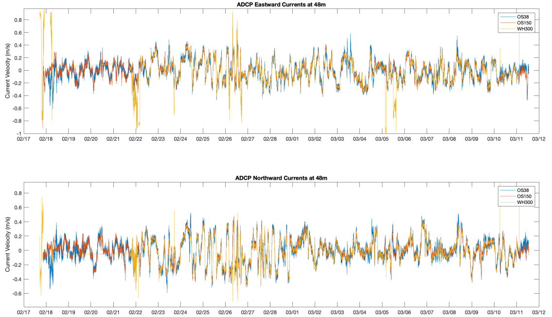
Figure 3: Comparison plot of 48 m velocities measured by the three ADCPs shows generally good agreement.
