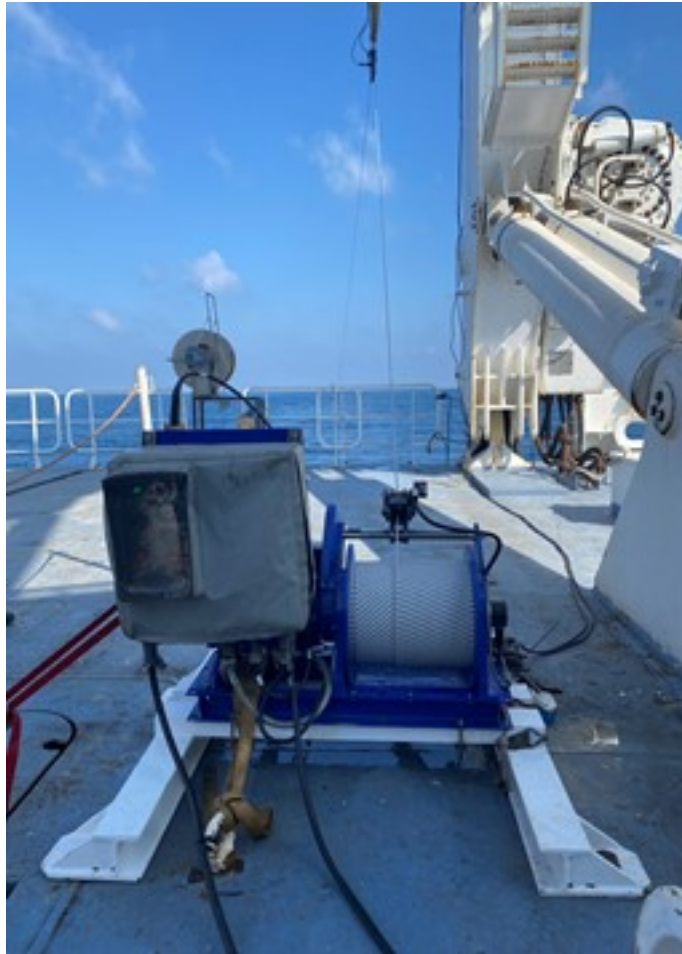
Figure 2: MVP Winch and Sheave
