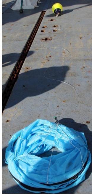
Figure 10: WHOI drifter: surface buoy (yellow), tether and drogue (blue).
