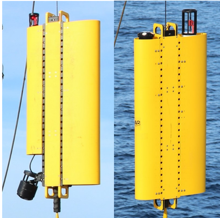
Figure 15: Wirewalker profilers fitted with RBR CTD and Nortek ADCP: downward-looking (left) and upward-looking (right).
