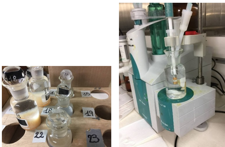
Figure 50: Dissolved oxygen samples and the Winkler titration instrument on board.
