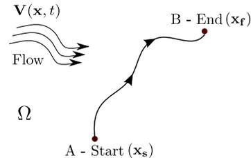
Fig. 1. Vehicle motion in time-varying flow field
