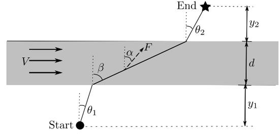
Fig. 3. Parameters involved in optimal crossing of a jet flow: jet speed  $V$  and width  $d$ ; Start (Circle), End (Star), distances from jet  $y_1, y_2$ ; vehicle speed  $F$  and headings  $\theta_1, \theta_2, \alpha$ ; resultant trajectory  $\beta$ .
