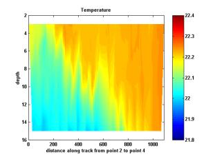
**Figure 14** Temperature measurement by the AUV between the endpoints of the track in Fig. 13. Temperature values are interpolated between upward and downward profiles. The apparent oscillation of the front is an artifact caused by different sensor response times.
