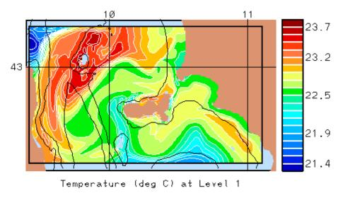
**Figure 21** Surface temperature after 4 days of model run on 26 September. Overlaid on the temperature field are the 50, 200 and 500m isobaths.
