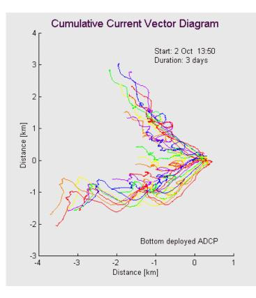
**Figure 12** Current measurement at the north coast of Elba. For each 30cm depth interval (bin), current vectors measured by an Acoustic Doppler Current Profiler are accumulated. Curves of bins close to the surface point to WSW, close to the bottom to NW.
