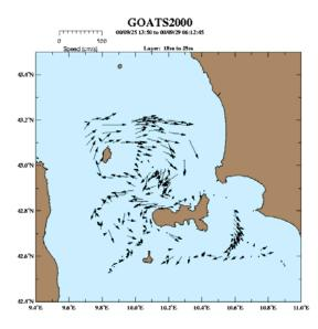
**Figure 10** *Currents measured by NRV Alliance with the ship-borne ADCP during the first update surveys. Data of 4 consecutive nights are merged. The SE current in the south-eastern corner is due to high wind force.*
