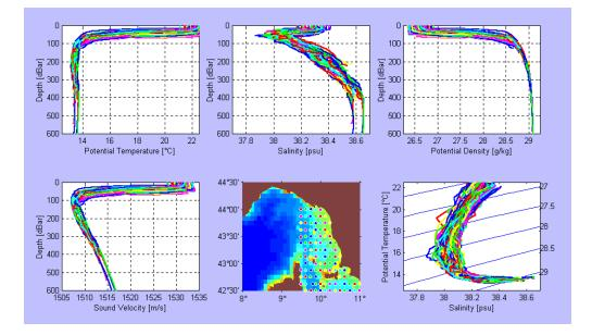
**Figure 5** *CTD stations of the initialisation survey. Profiles of salinity, density anomaly and sound velocity are calculated from measured parameters. The two branches in salinity below 400m mark the difference between Ligurian and Tyrrhenian Sea intermediate water.*
