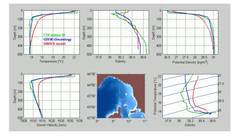
**Figure 7** A measured CTD profile (note the red dot on the map) at the southern survey boundary in the Tyrrhenian Sea compared with a mean profile from climatology. Climatology does not reflect the higher salinity in Thyrrhenian Sea intermediate water. Also shown is a profile from an operational navy model run, which was used a boundary condition for the CU-POM model.
