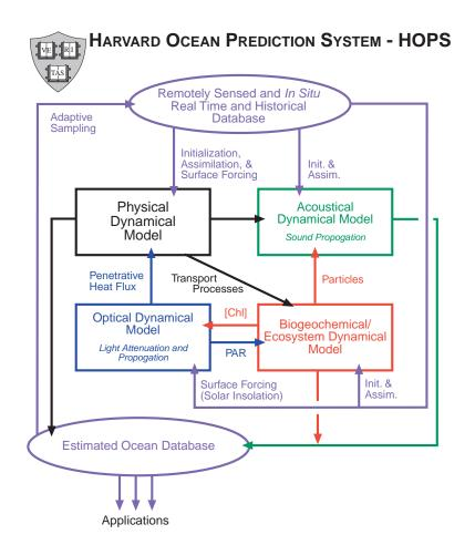
Figure 2 The Harvard Ocean Prediction System (HOPS).
