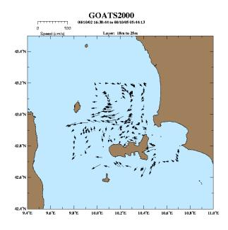
**Figure 11** *Currents measured by NRV Alliance with the ship-borne ADCP during update surveys in early October. The anti-cyclonic eddy has shifted towards the north.*
