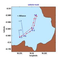
**Figure 13** Track of an autonomous underwater vehicle (AUV) north of Elba. The AUV samples temperature and salinity while it ascends and descends along its track. At the positions marked with an asterisk the AUV surfaces and updates navigation by the global positioning system (GPS).
