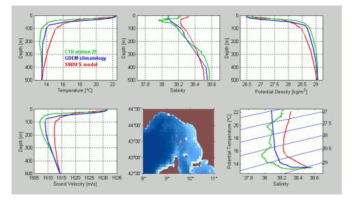
**Figure 6** A measured CTD profile (note the red dot on the map) at the western survey boundary in the Ligurian Sea compared with a mean profile from climatology. The transitional water between 50 and 300m depth is significantly colder than climatology. Also shown is a profile from an operational navy model run, which was used a boundary condition for the CU-POM model.
