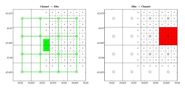
**Figure 16** 2-way nesting for modelling domains. (left) Channel to Elba (coarse to fine), (right) Elba to Channel (fine to coarse).
