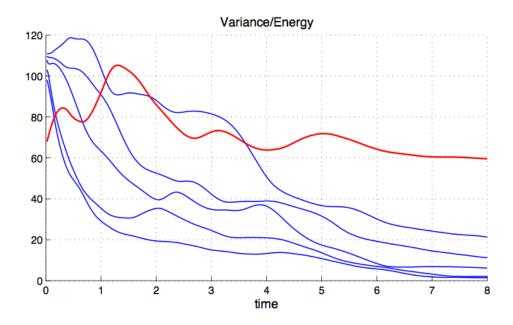
Figure 5-19: Evolution of principal variances  $\sigma_i^2(t)$ , i = 1, ..., 5 (blue curves) and mean field energy (red curve) for the flow behind a disk.
