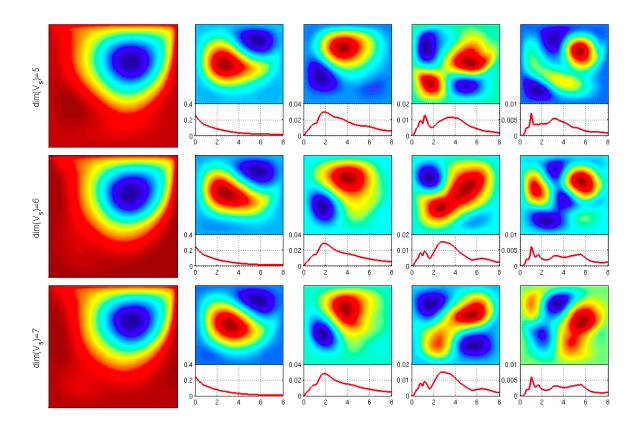
Figure 5-15: Left column: mean flow for various stochastic dimensionalities dim  $(\mathbf{V}_S)$  at t = 8. The four right columns on the right show the four most energetic modes  $\mathbf{u}_i(\mathbf{x}, t)$  in terms of their streamfunction as well as their associated variance  $E^{\omega}\left[Y_i^2(t;\omega)\right]$  as a function of time.
