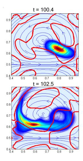
Figure 6-14: Concentration field for finite size particles (heavy particles) for two different time instants. The blue lines indicate streamlines for the mean flow. The red lines indicate clustering manifolds for the stochastic flow field.
