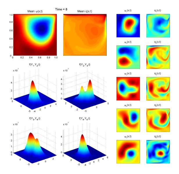
Figure 5-6: Mean field and basis of the stochastic subspace  $V_S$  in terms of the streamfunction and vorticity field; two-dimensional marginals of the five dimensional joint pdf  $f(\mathbf{y}, t)$  at time t = 8.
