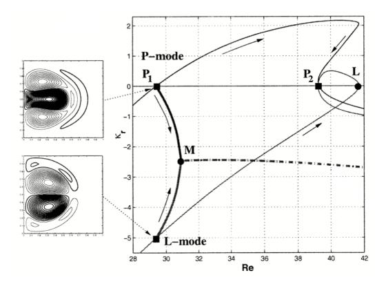
Figure 5-24: Spectral behavior of the eigenmodes involved into the various bifurcations of the anitsymmetric branch for the barotropic QG model (from Simonnet and Dijkstra [133]).
