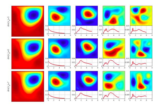
Figure 5-14: Left column: mean flow for various stochastic dimensionalities dim  $(\mathbf{V}_S)$  at t = 6. The four right columns on the right show the four most energetic modes  $\mathbf{u}_i(\mathbf{x}, t)$  in terms of their streamfunction as well as their associated variance  $E^{\omega}\left[Y_i^2(t;\omega)\right]$  as a function of time.
