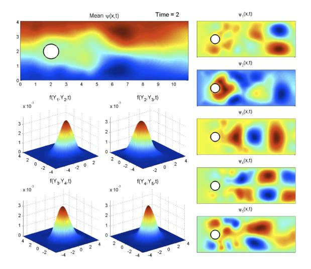
Figure 5-20: Mean field and basis of the stochastic subspace  $V_S$  in terms of the streamfunction; two-dimensional marginals of the five dimensional joint pdf  $f(\mathbf{y}, t)$  at time t = 2.
