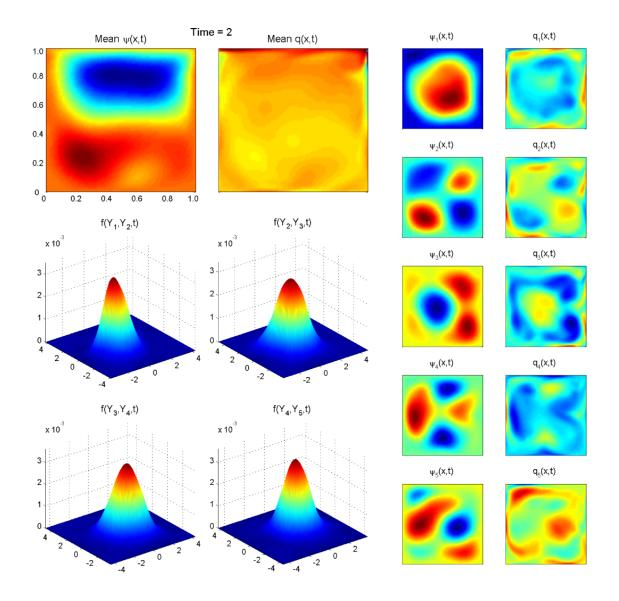
Figure 5-5: Mean field and basis of the stochastic subspace  $V_S$  in terms of the streamfunction and vorticity field; two-dimensional marginals of the five dimensional joint pdf  $f(\mathbf{y}, t)$  at time t = 2.
