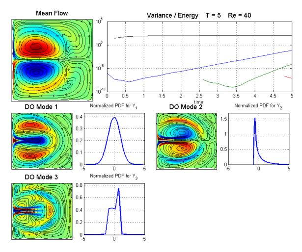
Figure 5-32: Stochastic response for Re = 40. Note that the first mode has symmetric spatial properties which are accompanied by symmetric pdf while the second mode has antisymmetric spatial properties with non-symmetric pdf.
