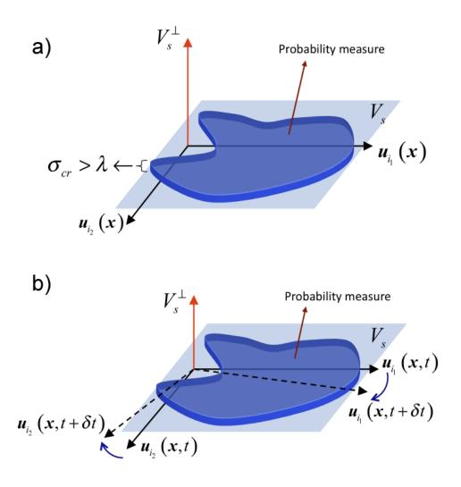
Figure 3-1: a) The stochastic subspace  $\mathbf{V}_{S}$  spanned by fields  $\mathbf{u}_{i}(\mathbf{x}, t)$  that corresponds to important variance. b) The variation of the  $\mathbf{u}_{i}(\mathbf{x}, t)$  inside  $V_{s}$  can always be covered by a rotation of the stochastic coefficients  $Y_{i}(t; \omega)$ .
