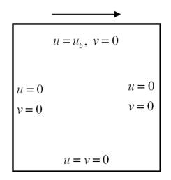
Figure 5-2: Driven cavity flow, problem configuration.
