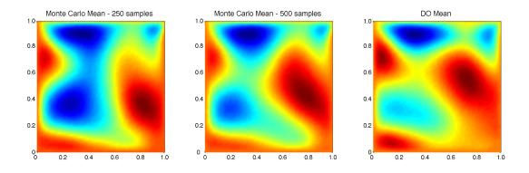
Figure 5-7: Mean velocity field (streamfunction) computed using Monte-Carlo method (250 and 500 samples) and the DO field equations (s = 5 modes) at t = 1.
