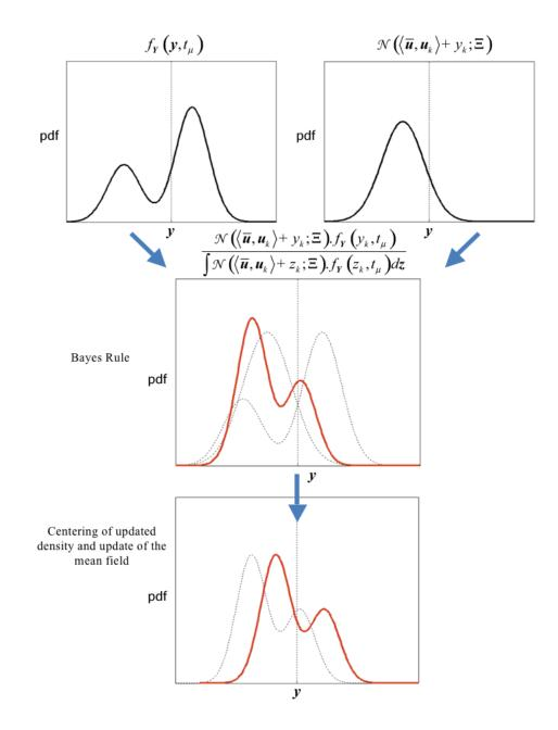
Figure 4-3: Update of the probability density function  $f_{\mathbf{Y}}(\mathbf{y},t)$  using data or measurements.
