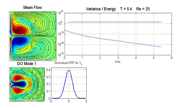
Figure 5-25: Stochastic response of the QG model for Re = 25. The left top plot shows the mean flow in terms of the vorticity (colormap) and the streamlines (black solid curves). The right-top plot indicates the energy of the mean flow (red curve) and the variance of the stochastic mode. The bottom plot indicates the first DO mode together with the pdf for the stochastic coefficient.
