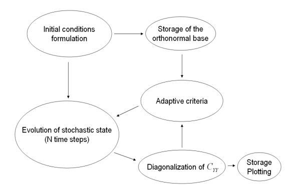
Figure B-1: Computational algorithm for the adaptive DO equations.
