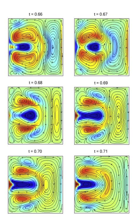
Figure 5-27: Oscillation of the DO mode during convergence to the steady state attractor for Re = 35.
