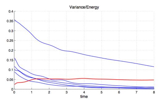
Figure 5-4: Evolution of principal variances  $\sigma_i^2(t)$ , i = 1, ..., 5 (blue curves) and mean field energy (red curve) for the flow in a cavity.
