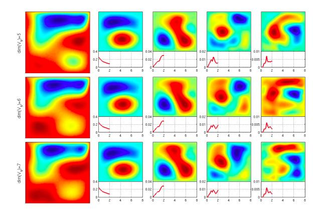
Figure 5-13: Left column: mean flow for various stochastic dimensionalities dim  $(\mathbf{V}_S)$  at t = 2. The four right columns on the right show the four most energetic modes  $\mathbf{u}_i(\mathbf{x}, t)$  in terms of their streamfunction as well as their associated variance  $E^{\omega}\left[Y_i^2(t;\omega)\right]$  as a function of time.
