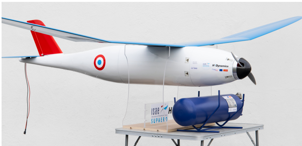
Figure 3: The Mermoz drone in the version integrating a 7L liquid dihydrogen tank.
