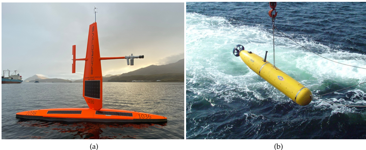
Figure 5: (a) An example of an autonomous sailing vessel (Source: NOAA and Saildrone Inc.). (b) An example of an AUV (Source: Bluefin Robotics).
